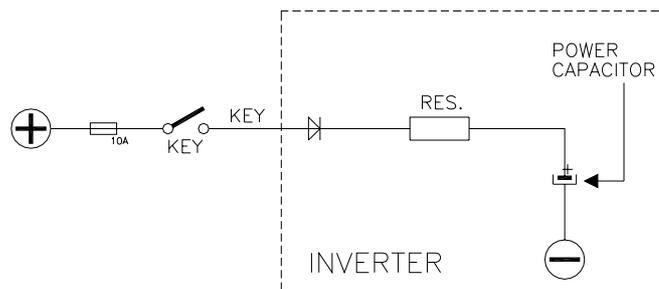
When the key is switched ON, the inverter tries to charge the capacitors through a power resistance and check if the capacitors are charged within a timeout. If this is not true: an alarm is signalled; the main contactor is not closed.
