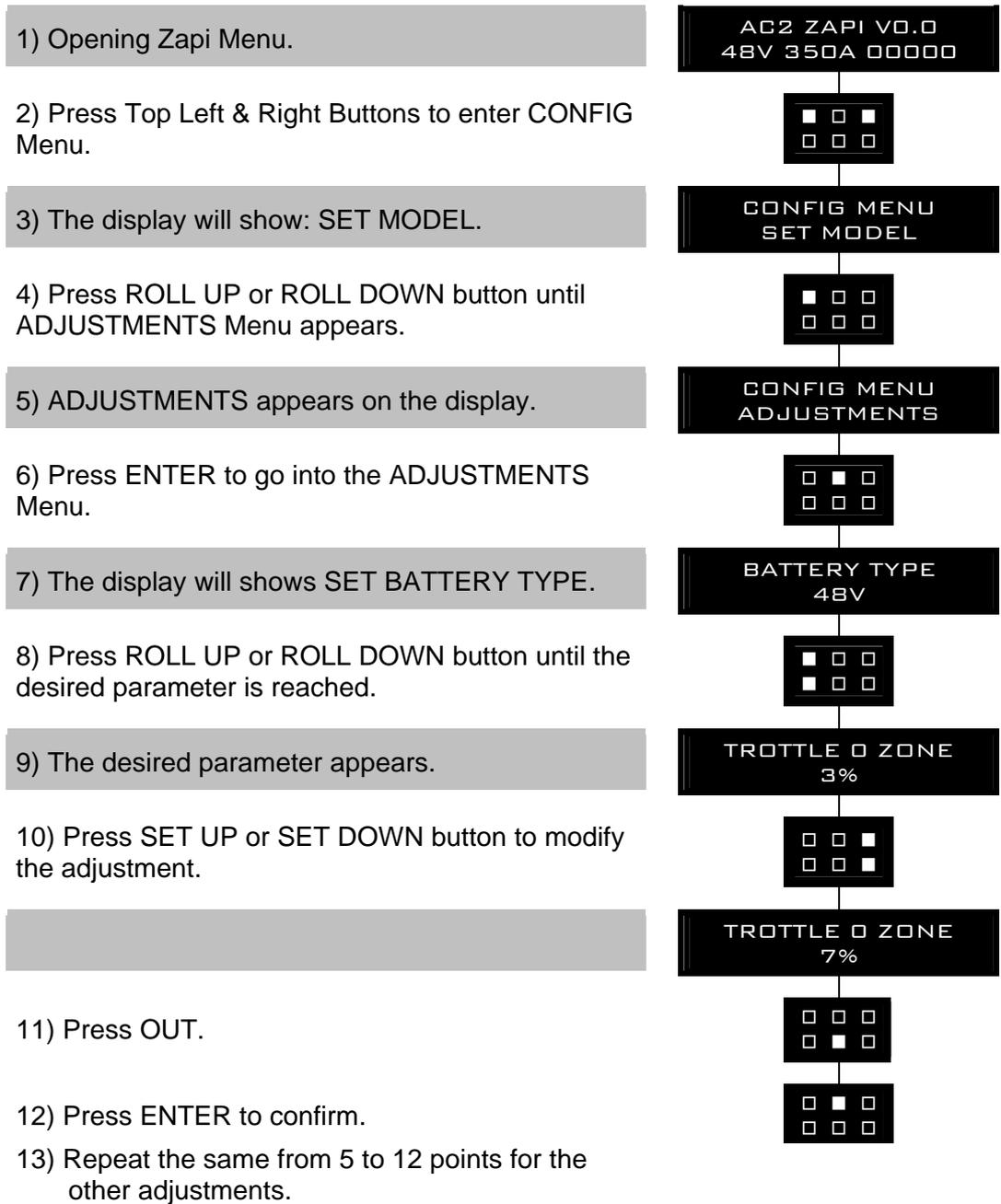
Flow chart showing how to use the SET BATTERY TYPE adjustment.
