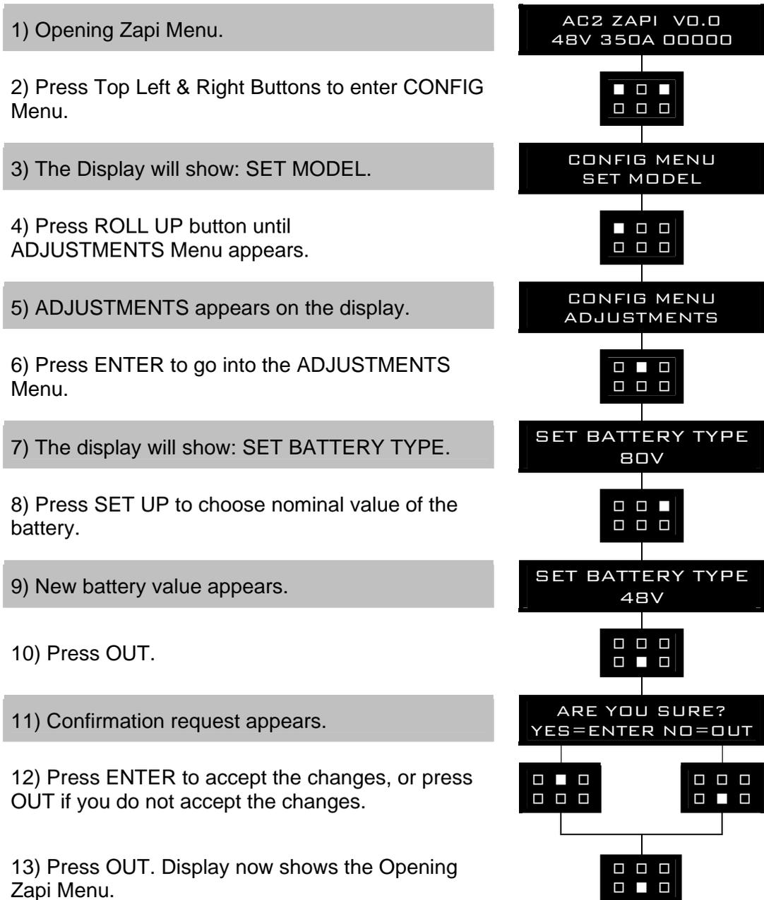
Flow chart showing how to carry out ADJUSTMENT BATTERY operation by console.
