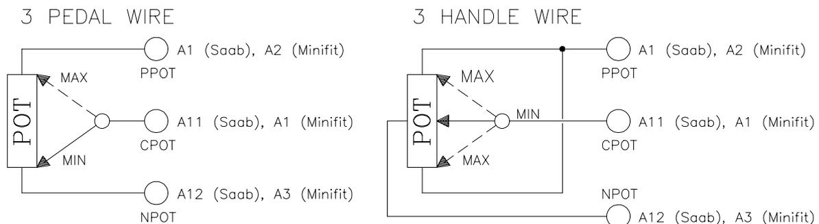
The Procedure for automatic potentiometer signal acquisition is carried out using the Console. This enables adjustment of the minimum and maximum useful signal level (PROGRAM VACC function), in either direction. This function is unique when it is necessary to compensate for asymmetry with the mechanical elements associated with the potentiometer, especially relating to the minimum level.
