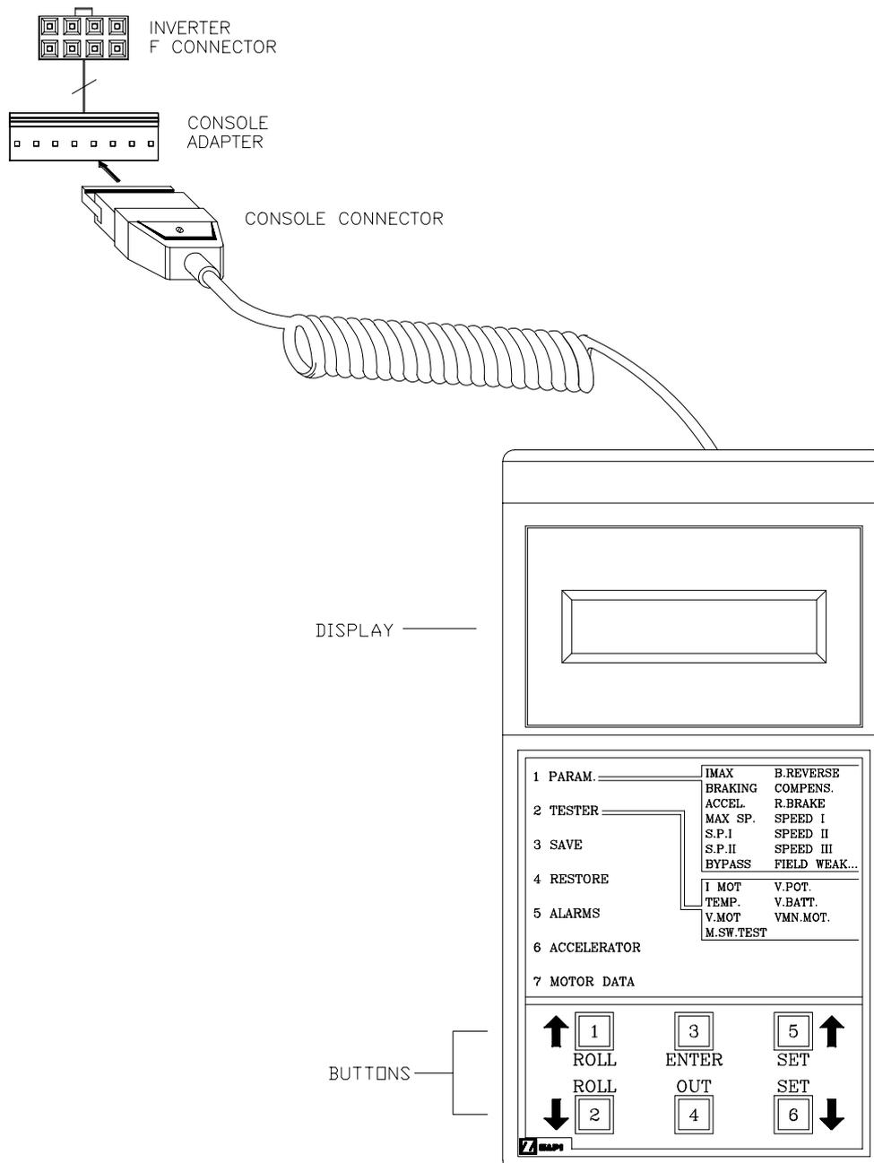
Digital consoles used to communicate with AC inverter controllers must be fitted with EPROM CK ULTRA, minimum "Release Number 3.02".
