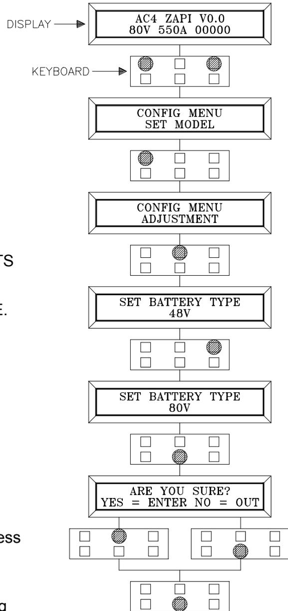
Flow chart showing how to carry out ADJUSTMENT BATTERY operation by console.
