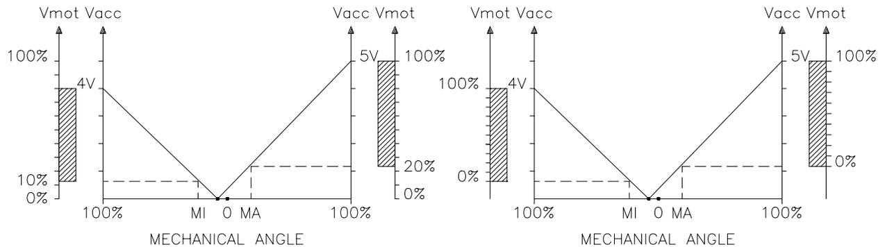
The two graphs show the output voltage from a non-calibrated potentiometer with respect to the mechanical “zero” of the control lever. MI and MA indicate the point where the direction switches close. 0 represents the mechanical zero of the rotation. The Left Hand graph shows the relationship of the motor voltage without signal acquisition being made. The Right Hand Graph shows the same relationship after signal acquisition of the potentiometer.
