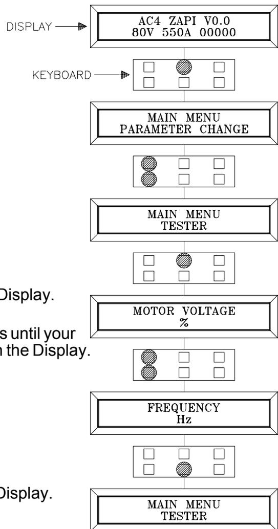
Remember it is not possible to make any changes using TESTER. All you can do is measure as if you were using a pre-connected multimeter.
