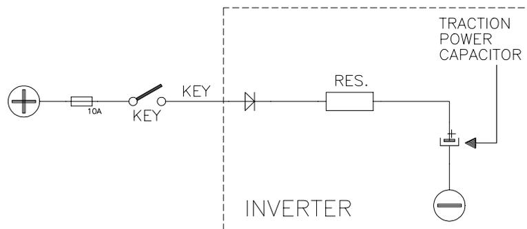
When the key is switched ON, the inverter tries to charge the capacitors through a power resistance and check if the capacitors are charged within a timeout. If this is not true: an alarm is signalled; the main contactor is not closed.
