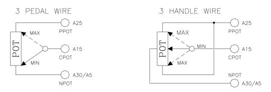
The Procedure for automatic potentiometer signal acquisition is carried out using the Hand Set. This enables adjustment of the minimum and maximum useful signal level, in either direction.
