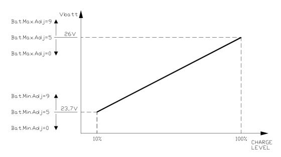
The Battery Charge detection follows this algorithm:
