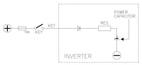
When the key is switched ON, the inverter tries to charge the power capacitors through a power resistance, and check if the capacitor are charged within a timeout. If they do not charge, an alarm is signalled; the main contactor is not closed.
