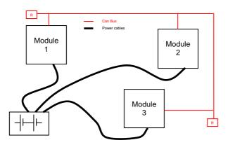
The red lines are can wires.
