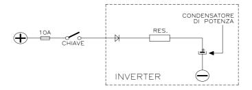
When the key is switched ON, the inverter tries to charge the capacitor through a power resistance, and check if the capacitor are charged within a timeout. If they do not charge, an alarm is signalled; the main contactor is not closed.
