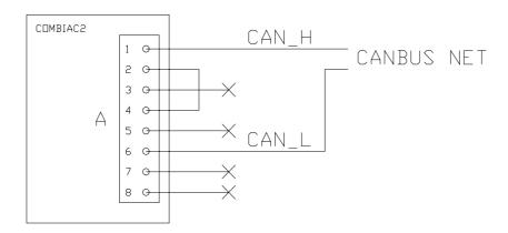
Bridge 2-4 connects one built-in 120 ohm can termination resistance, the second will be connected in another module of the canbus net.
