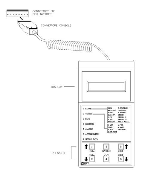
Digital consoles used to communicate with AC inverter controllers must be fitted with EPROM CK ULTRA, minimum "Release Number 3.02".
