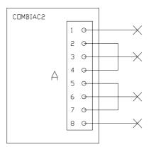
Bridge 2-4 and 5-7 connect both built-in120 ohm can termination resistances.
