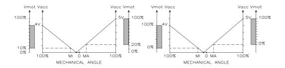
The two graphs show the output voltage from a non-calibrated potentiometer with respect to the mechanical "zero" of the control lever. MI and MA indicate the point where the direction switches close. 0 represents the mechanical zero of the rotation.
