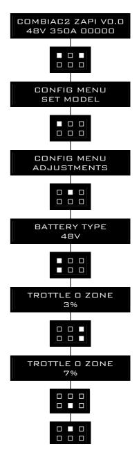
Flow chart showing how to use the SET BATTERY TYPE adjustment.
