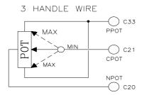
The Procedure for automatic potentiometer signal acquisition is carried out using the Console. This enables adjustment of the minimum and maximum useful signal level
