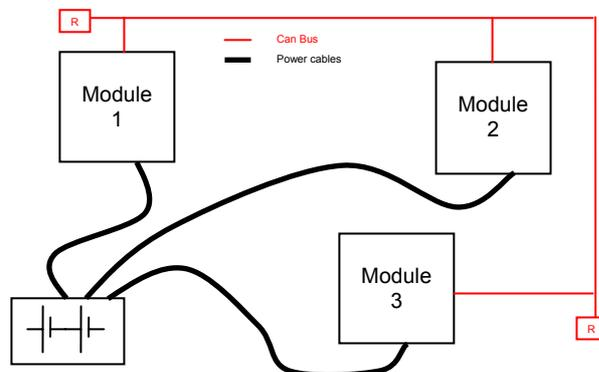
The red lines are can wires.
