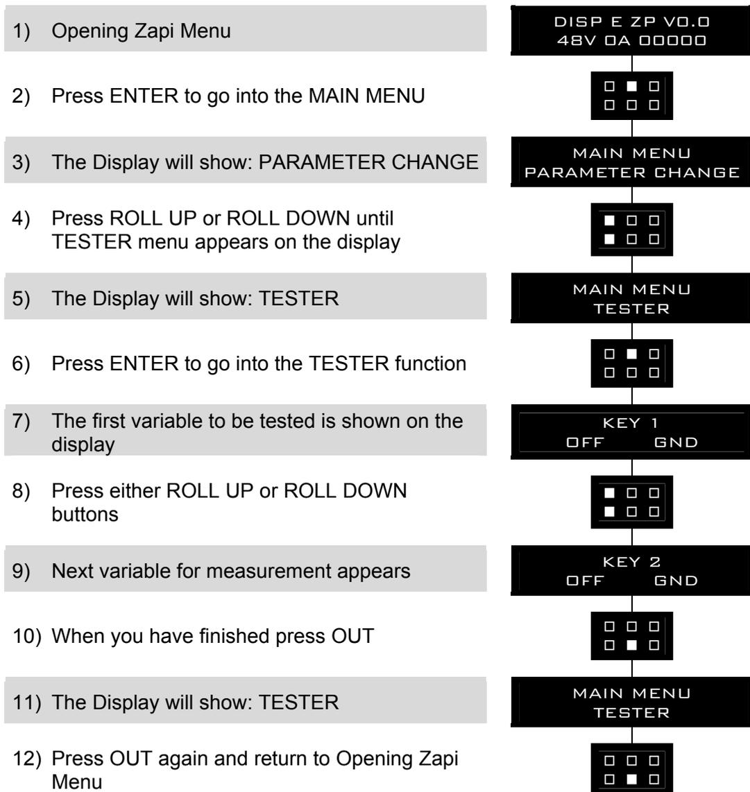
Remember it is not possible to make any changes using TESTER. All you can do is measure as if you were using a pre-connected multimeter.
