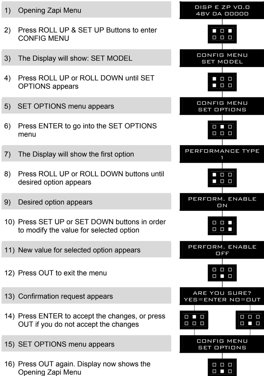
Flow chart showing how to make Program changes using Digital Console:
