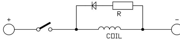
R resistor value shall be about the same of coil resistance value; power level is to be computed as follows:
