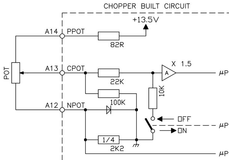
PEDAL TYPE = ON range 0.6 to 10V.
