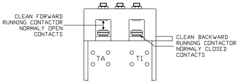
It could be necessary changing both contactors.
