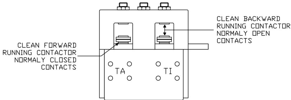
It could be necessary changing both contactors.
