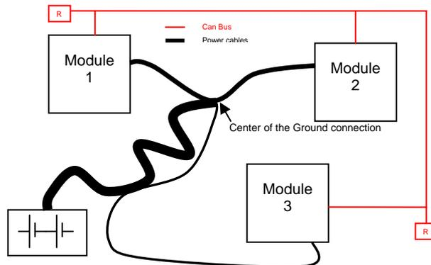
**Note: Module 1 power  $\approx$  Module 2 power > Module 3 power**
