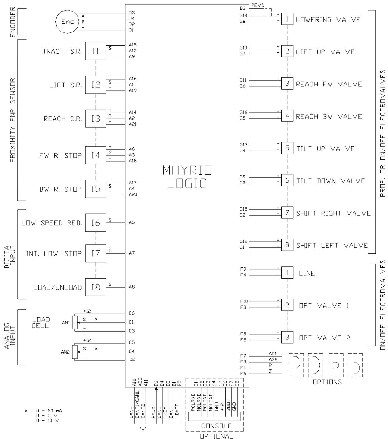
PAUX (B6) = SUPPLY FOR ELECTROVALVES CAN BE +BATTERIE OR 24VOLT.
