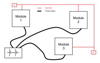
The red lines are can wires.
