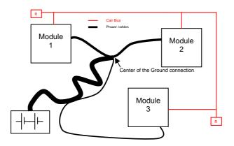
Note: Module 1 power ≈ Module 2 power > Module 3 power
