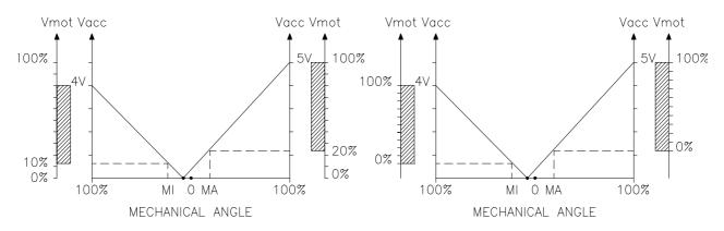
The above graphs show the output voltage of a potentiometer that has not been calibrated compared to the mechanical "zero" of the tiller knob (MI and MA indicate the closing points of the microswitches, 0 represents the mechanical angle of rotation of the throttle). The first graph shows the corresponding motor voltage without acquisition; the second graph shows the corresponding voltage after potentiometer signal acquisition.
