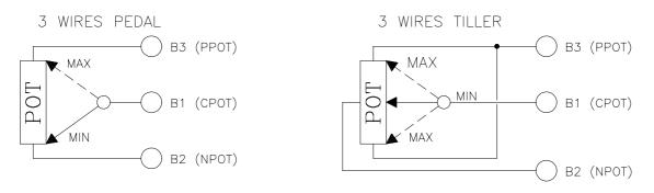
Automatic minimum and maximum signal acquisition must be carried out (PROGRAM VACC function) using the programming console and in both directions. This function is indispensable when compensating an eventual asymmetry in the mechanical components of the potentiometer and for minimum level adjustment in particular.
