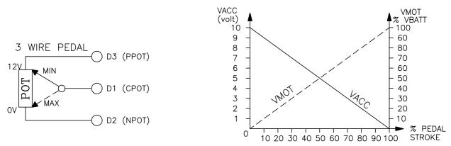
VACC = accelerator signal voltage on pin D1; VMOT = percentage on battery voltage on the motor.
