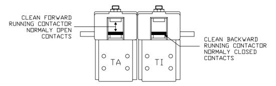
It could be necessary to change both contactors.
