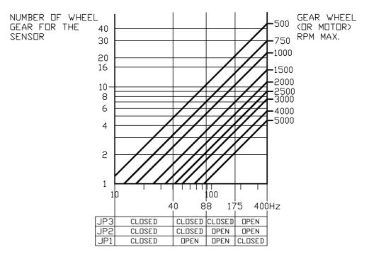
Example: The requests are revolutions 2500 RPM max and on the drive shaft is connected with a 4 - gear wheel. For the selection of the jumpers positions point from the scheme where the 2500 rpm line crosses the 4 - gear line, then modify the jumpers like as in the table under the scheme; in our case it has to be used the table from 88 kHz to 175 kHz.
