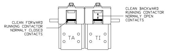
It could be neccessary to change both contactors.
