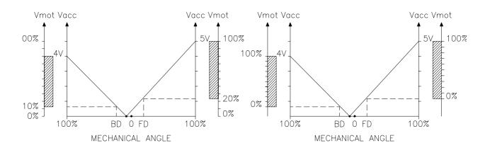
The two graphs show the output voltage from a non-calibrated potentiometer with respect to the mechanical "zero" of the control lever. MI and MA indicate the point where the direction switches close. 0 represents the mechanical zero of the rotation. The Left Hand graph shows the relationship of the motor voltage without signal acquisition being made. The Right Hand Graph shows the same relationship after signal acquisition of the potentiometer.
