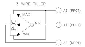
The Procedure for automatic potentiometer signal acquisition is carried out using the Console. This enables adjustment of the minimum and maximum useful signal level (PROGRAM VACC function), in either direction. This function is unique when it is necessary to compensate for asymmetry with the mechanical elements associated with the potentiometer, especially relating to the minimum level.
