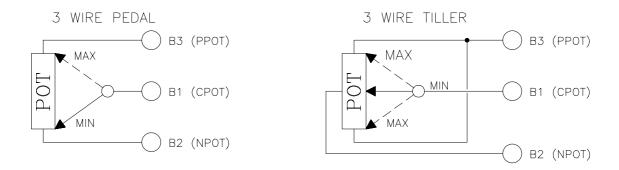
The Procedure for automatic potentiometer signal aquisition is carried out using the Console. This enables adjustment of the minimum and maximum useful signal level (PROGRAM VACC function), in either direction. This function is unique when it is necessary to compensate for asymmetry with the machanical elements associated with the potentiometer, especially relating to the minimum level.
