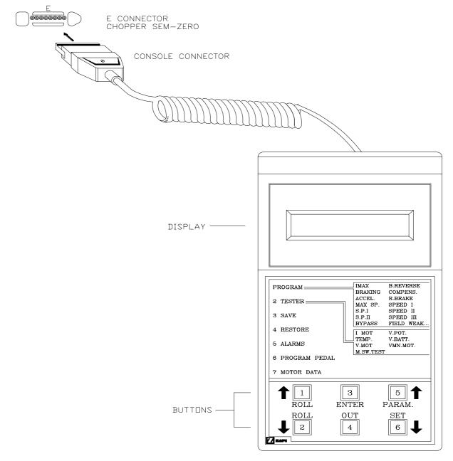
Digital Consoles used to communicate with SEM-Zero choppers must be fitted with Eprom CK ULTRA.
