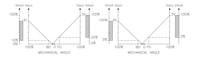
The two graphs show the output voltage from a non-calibrated potentiometer with respect to the mechanical "zero" of the control lever. MI and MA indicate the point where the direction switches close. 0 represents the mechanical zero of the rotation. The Left Hand graph shows the relationship of the motor voltage without signal aquisition being made. The Right Hand Graph shows the same relationship after signal aquisition of the potentiometer.
